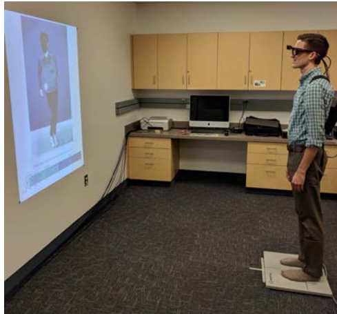
Figure 3: Setup of the experiment: Shown is one participant wearing the eye-tracking device and standing on the force plate while looking at a posture projected onto the wall.
