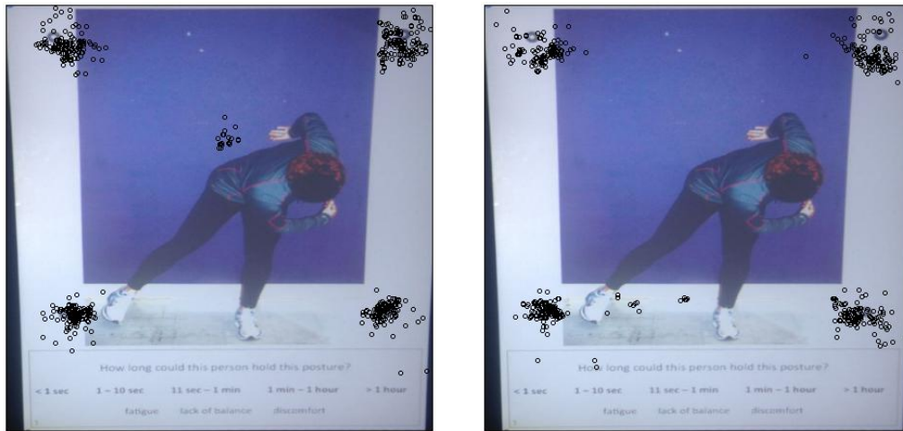
Figure 4: Scatterplot showing the focus points, confirming the proper calibration of the eye-tracking device at the start of the experiment (left) and end of the experiment (right) for Participant 1.
